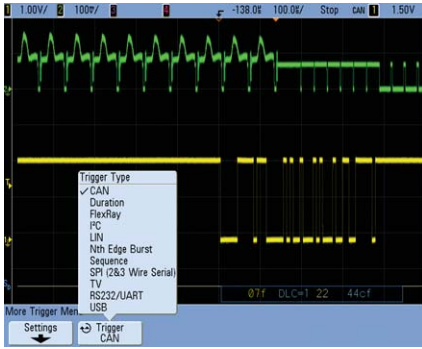
Trigger on and decode CAN serial packets.
